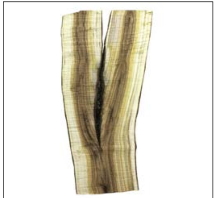
Trees with codominant leaders are more likely to split during storms. Note the decay present in branch union.
